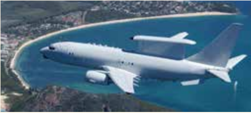
The MESA radar provides air-to-air coverage, air-to-surface coverage.
